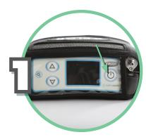
Turn off the X-PLO<sub>2</sub>R<sup>™</sup> by pressing the power button for 2 seconds.
