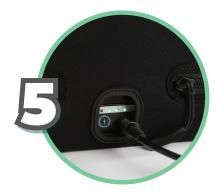
Connect charged battery to the X-PLO<sub>2</sub>R.
