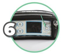
Turn on the X-PLO₂R by pressing the power button for 2 seconds. Set the flow setting to your prescribed setting and use normally.
