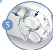
5 Press the latch button with thumb or finger and pull the column out of the concentrator using the pull ring attached to the bottom of the column cap.
