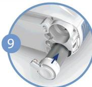
9 Insert the new column into the concentrator. Do not leave the column exposed after the dust caps are removed; it should be inserted into the concentrator immediately to minimize environmental exposure.
