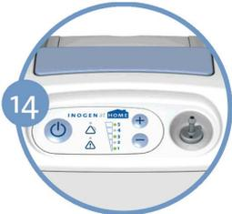
14 Press and hold the plus button for ten seconds. Flow indicators 1, 3 & 5 will be illuminated and columns will be reset. Release the plus button. Press the power button to turn on the concentrator and use normally.
